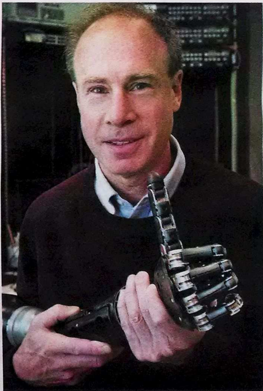
Andrew Schwartz (above), professor of neurobiology, and Michael L. Boninger, professor and chair of physical medicine and rehabilitation, are working with spinal cord injury patients to test a multifunctional prosthetic limb that is mounted on a wheelchair. The prostheses will be controlled by the patients' brains through implanted electrodes connected to a computer.
