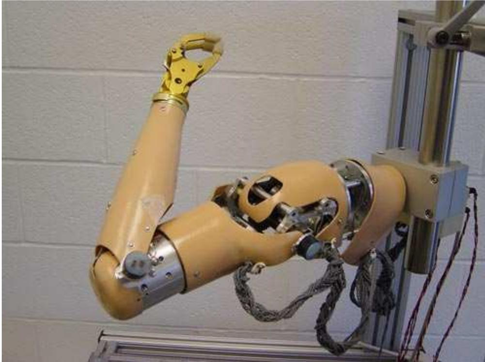
The prosthetic limb, the size of a child's arm, has working shoulder and elbow joints and is equipped with a simple gripper to grasp and hold food.
