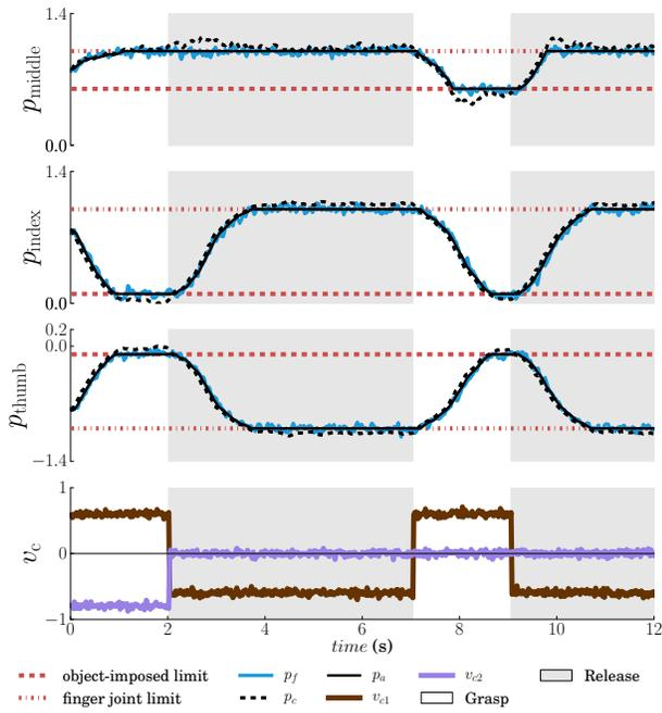
Fig. 5. Finger positions and low-DoF command velocities during simulated grasping of a slot object
